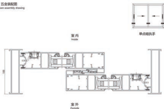
五金装配图 Hardware assembly drawing
